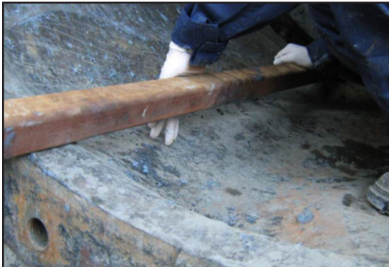
Severity of wear on ID of trunion housing
